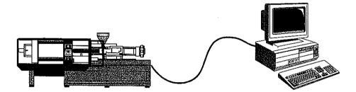
In its physical manifestation, the computer interface has been designed as serial interface and subset of standard V.24 (CCITT), or RS232C. A 9-pin sub-miniature D-socket, whose contacts are assigned as follows, has been mounted on the control cabinet of the MC4:
