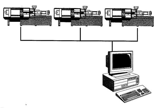
The **length of the cables** from and to the hub must not exceed **100 meters**. To obtain greater noise immunity, STP cables (Shielded Twisted Pair) should be used in preference to UTP cables (Unshielded Twisted Pair).
